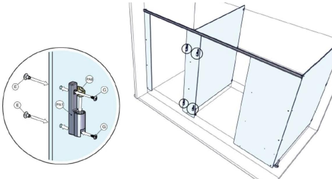
From there, assemble the remaining components, keeping the upper half of the hinge and its fixings aside for the moment. **HINGES CAN EITHER BE SET TO SELF-CLOSING OR MANUAL-CLOSING AS SHOWN BELOW.**
