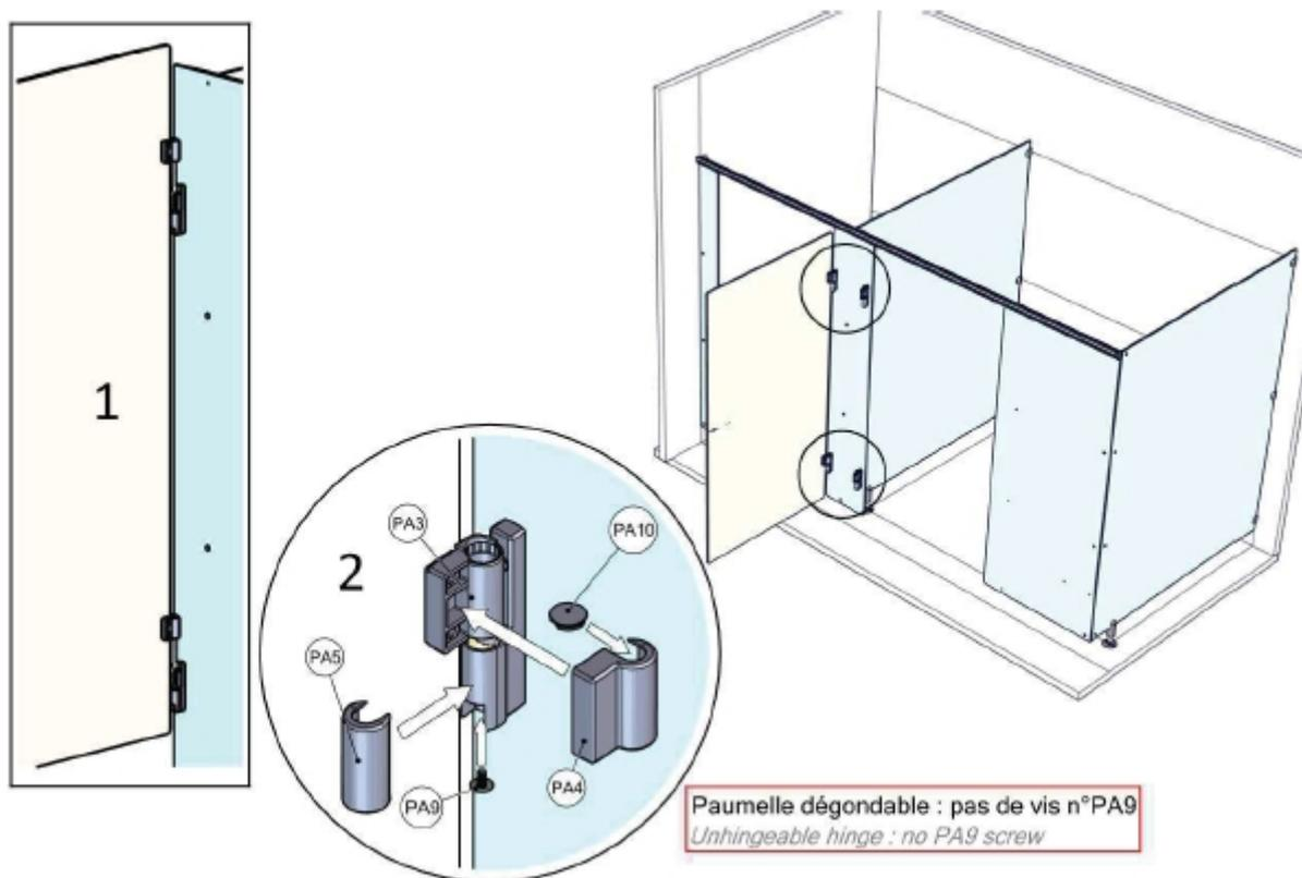
You can now place the door Hinge 'PA3' onto the Pilaster/Partition Hinge 'PA1' as shown below. Screw in Fixing 'G' and 'PA9' and tighten both until the hinge is securely locked together. Once this has been completed finish the Hinge by covering both the upper and lower halves with the Hinge Cover Plate 'PA4' and 'PA5'.
