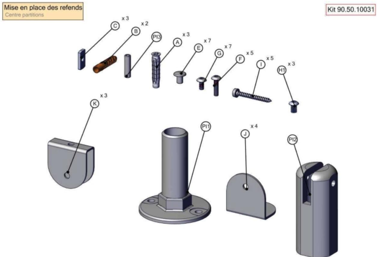
Fix the 3 Wall Brackets 'K' where you've marked the cubicle centre lines and place the foot in the partition foot position. **PLEASE DO NOT FIX THE FOOT IN PLACE AT THIS POINT AS YOU MAY NEED TO MAKE ADJUSTMENTS LATER.**
