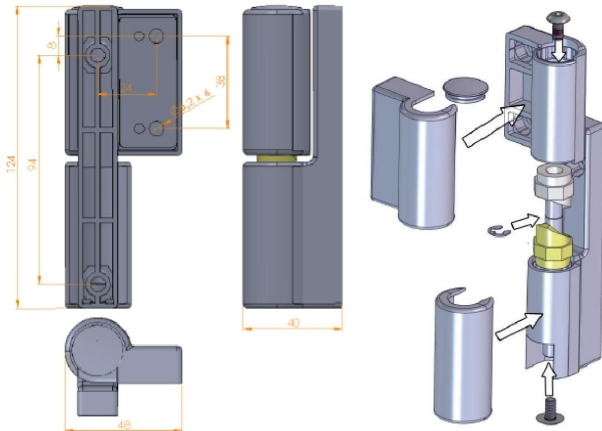
For doors shown on the Job Specific drawings as **PARTITION** mounted, fix the Hinge Packers 'PA11' and the lower half of the Hinge 'PA1' to the **PARTITION** as shown below using Fixing 'E' and 'G'.
