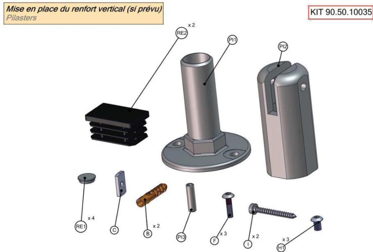
The **PILASTERS** have pre-drilled holes, line up the Stiffener Post with these holes and insert the 'F' Fixing into the top hole and the 'H1' Fixings into the lower 3 holes. Use the 'RE1' and 'RE2' Caps to finish as shown below
