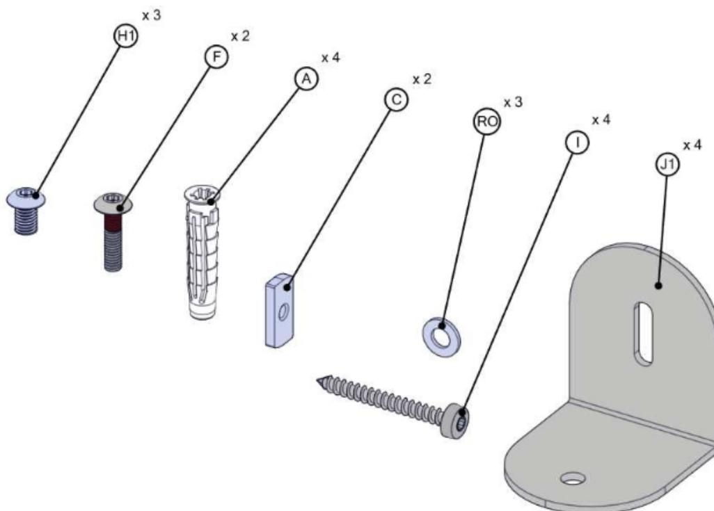
Using the pre-marked Pilaster to Wall position and Fixings 'A' and 'I', fix all the Side Wall Brackets 'J1' to the wall. Please note that the top and bottom bracket must be in line with the Pilaster panel.
